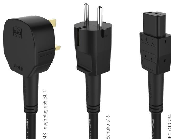
The plugs and connectors fitted to QED XT5 are standard high quality items such as the MK Tough Plug (used in military and health service applications) and as such have not been adulterated in any way by us. However, we do treat all the pins with contact cleaner to protect them from corrosion and enhance the quality of the electrical contact
