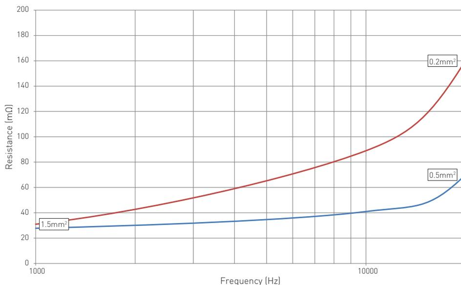
Figure 6. Graph of resistance versus frequency for QED power cables
