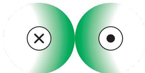
Figure 2. Proximity Effect in live & neutral conductors
